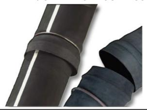
This layflat water discharge hose is built with a male and female end enabling the user to connect hoses. The male end is inserted into the female end and locked into place with a steel ring.
